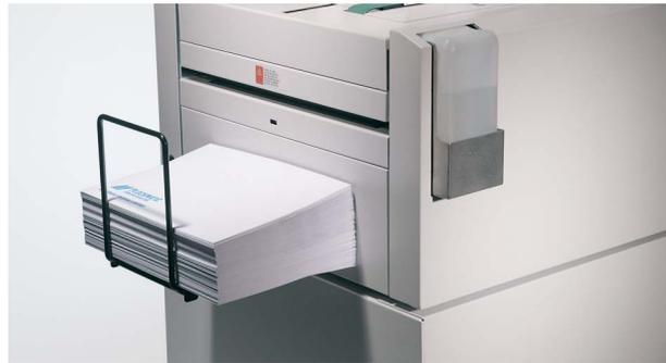
**Receiving Tray** The envelopes are counted and stacked on the receiving tray, ready to be franked and posted. Warning sensor notifies operator when the envelope stack needs to be emptied.
