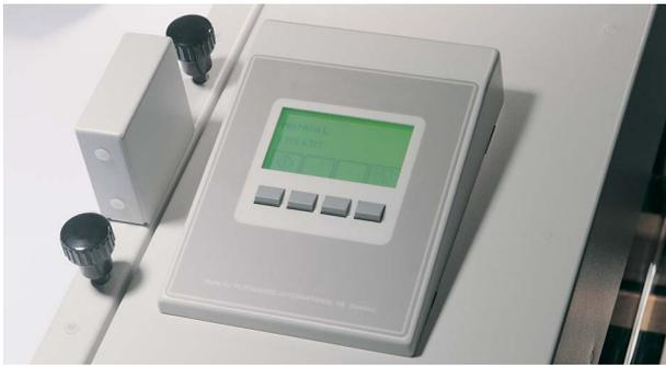
**Display** Extremely easy to set up for different jobs thanks to a fully microprocessor controlled operation. Just 4 buttons to do the settings. Step-by-step guidance of the operator through the different menus on the LCD display.
