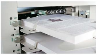
Loading. The open design makes it very easy to load the high capacity bins. Bins not in operation can easily be loaded while the others are running. With the various programming options the collator can then run continuosly without stops for reloading.
