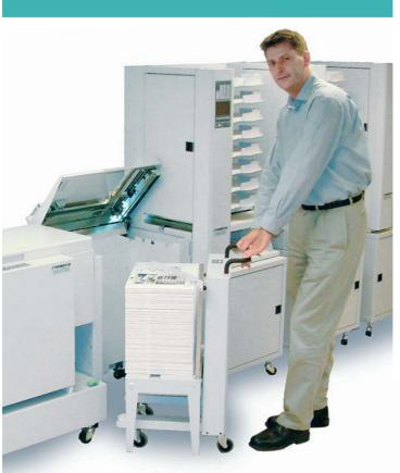
The Plockmatic 101 HCS DocuStack has full communication with the DocuVac 100 which means speed and paper size are automatically set. The integrated air venting system enables stacking of static material. When booklet making is required and the DocuBind 102 is a part of the system, there is no need to roll away the stacker – simply use the by-pass mode.
