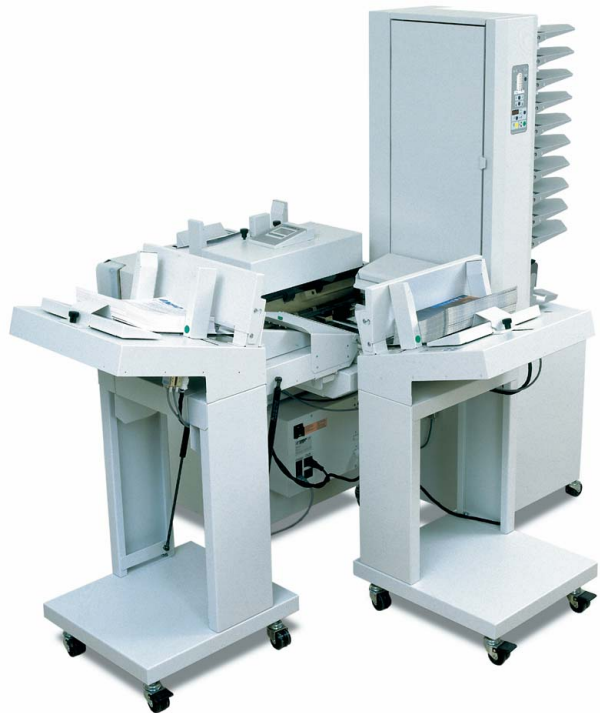
Three different feeders around the DocuMail. The Plockmatic 49-OMR sheet feeder, the Plockmatic 46 booklet feeder and the Plockmatic 310+ multi bin feeder. This configuration handles personalised mailings including up to 10 different brochures, one catalogue and your customised sales letter.
