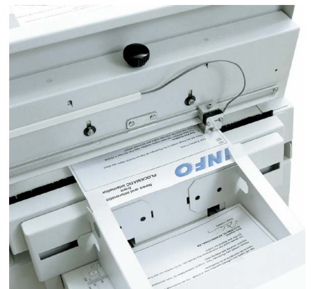
Three different feeders around the DocuMail. The Plockmatic 49-OMR sheet feeder, the Plockmatic 46 booklet feeder and the Plockmatic 310+ multi bin feeder. This configuration handles personalised mailings including up to 10 different brochures, one catalogue and your customised sales letter.
