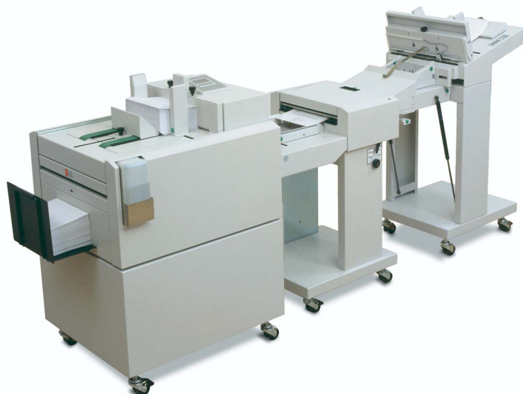
A typical system configuration with a PL49 SheetFeed, PL51 SetFold and the PL45 DocuMail inserter. Groups are assembled in the PL 49, either by OMR or by presettable counter. The complete groups are nest folded by PL51 and subsequently inserted and sealed by the PL45 inserter.
